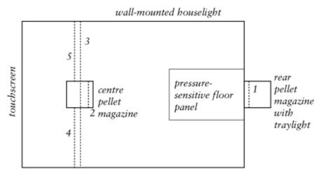
Infrared beams: (1) rear magazine; (2) centre magazine; (3) centre locomotor beam; (4) left locomotor beam; (5) right locomotor beam.
